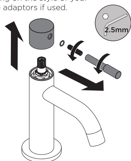
**Unscrew peg lever by hand**, then remove the threaded rod with hex key.
