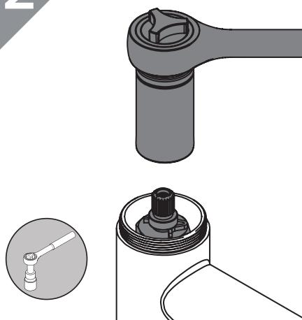
Remove the valve using the tool required for your tap. Check any seals and O-rings for damage. Replace valve if necessary.
