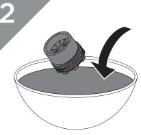
Check all loose parts for damage and then soak using a suitable solution to de-scale.
