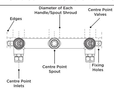
Take note of the following dimensions when fitting, or mark on the fitting location where needed.
