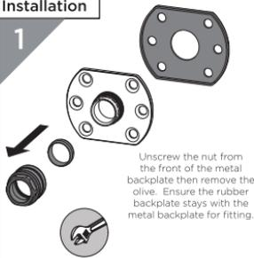
Unscrew the nut from the front of the metal backplate then remove the olive. Ensure the rubber backplate stays with the metal backplate for fitting.
