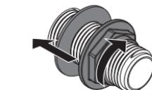
Slide the washer towards the wall and tighten the backnut.
