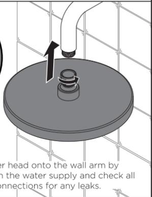
Screw the shower head onto the wall arm by **HAND ONLY**. Turn on the water supply and check all joints and connections for any leaks.
