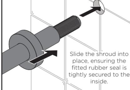
Slide the shroud into place, ensuring the fitted rubber seal is tightly secured to the inside.
