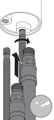
Thread the tap and tails through the plinth ensuring the rubber seal
