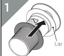
Thread the washer onto the waste until it is sitting tightly under the lip.
