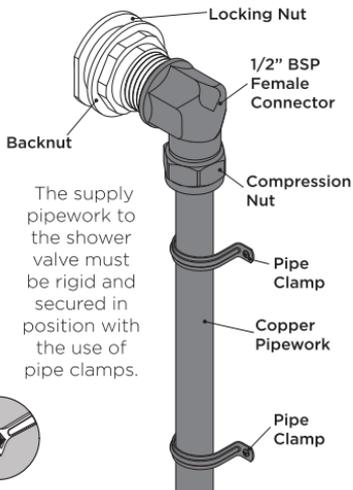
The supply pipework to the shower valve must be rigid and secured in position with the use of pipe clamps.
