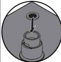
Ensure the filter washer is correctly inserted into the fixed head.
