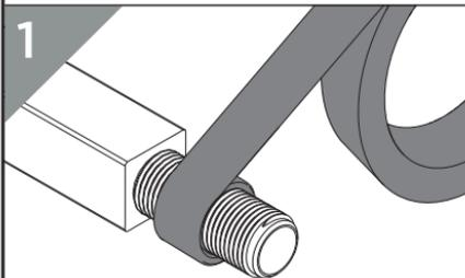
Use a suitable sealant that is compliant with UK Water Regulations around the thread.
