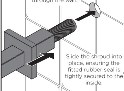
Slide the shroud into place, ensuring the fitted rubber seal is tightly secured to the inside.
