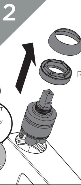
Remove the shroud and retaining nut and then lift the cartridge out of the tap.
