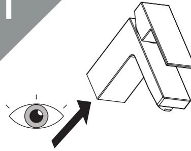
Look underneath the tap body to observe fixing kit rod(s) and tail inlet positions.
