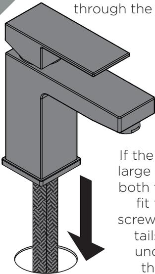
If the hole is not large enough for both tail ends to fit through, screw one of the tails in from underneath the basin.
