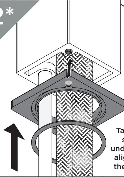
If required, thread the flexible tails and fixing kit rods through the plinth and rubber seal (if loose) and align with tap body.
