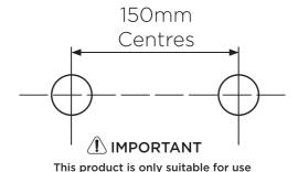
with 15mm copper pipework.
