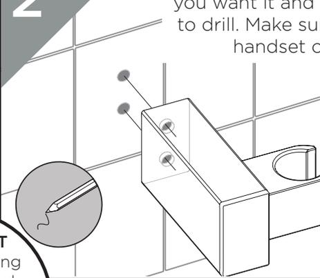
On most models, the screw holes are large enough to fit a pencil through for easy marking.
