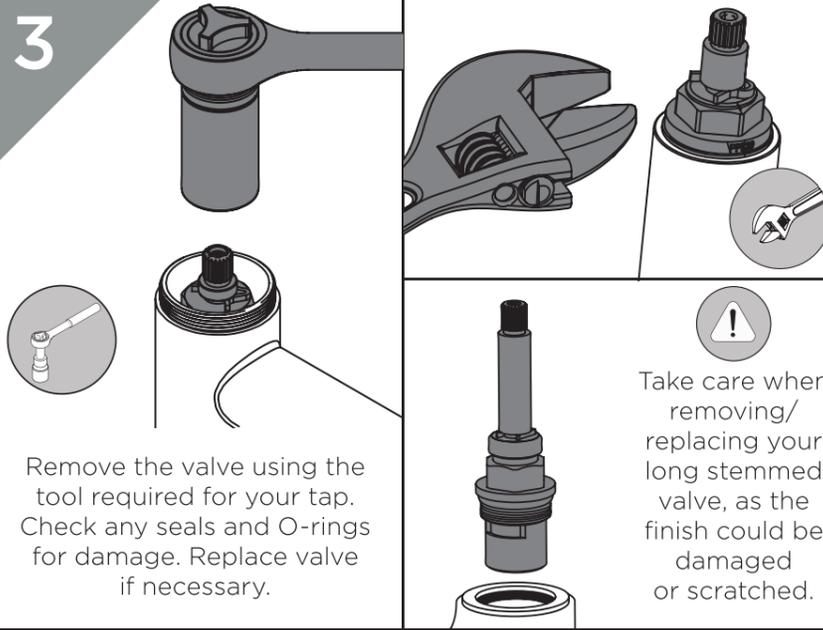
Remove the valve using the tool required for your tap. Check any seals and O-rings for damage. Replace valve if necessary.
