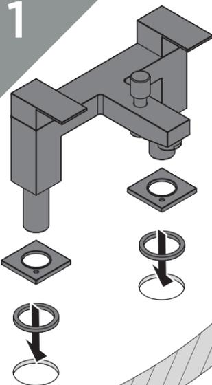
Feed the tap body through the plinths and ensure rubber plinth seals are in place
