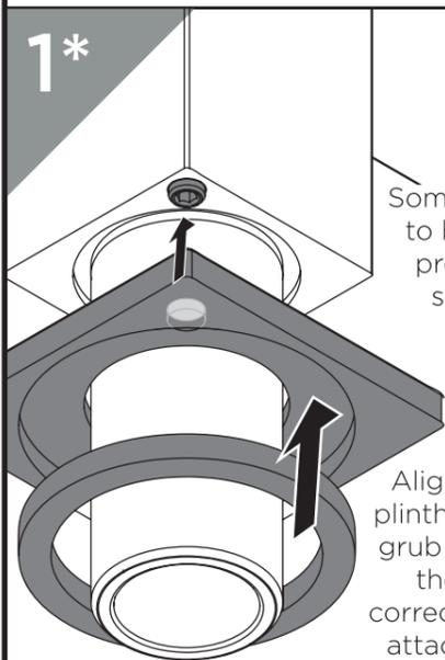
Some plinths will need to be aligned with a pre-attached grub screw in the tap
