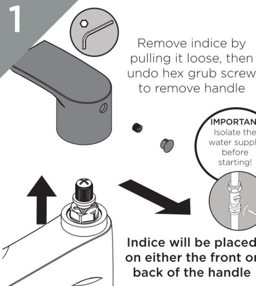
Remove indice by pulling it loose, then undo hex grub screw to remove handle
