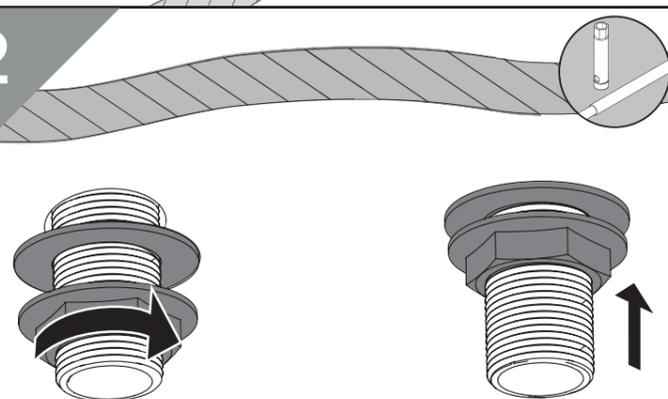
To secure the taps to the bath, use a box spanner to tighten the metal backnuts underneath ensuring the washer is correctly positioned in between the backnuts and the bath
