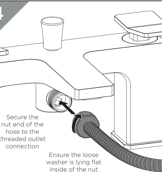
Secure the nut end of the hose to the threaded outlet connection
