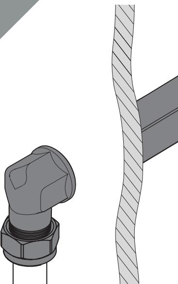
Use a tap connector (not included) to connect to the pipework. Connect the outlet pipework to your desired shower (not supplied) and to your wall arm.
