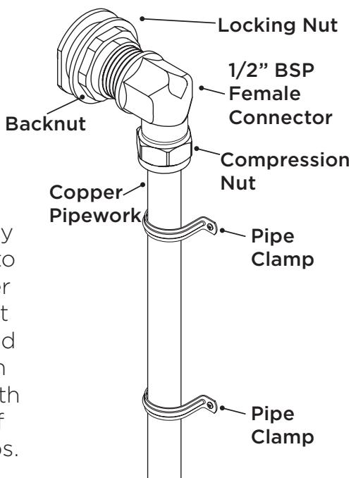
The supply pipework to the shower valve must be rigid and secured in position with the use of pipe clamps.
