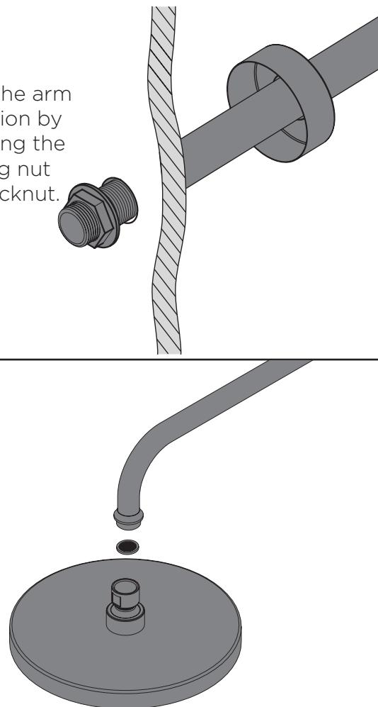
Screw your chosen shower rose onto the shower arm by **HAND ONLY**. Ensure the sealing washer is used where supplied. Turn on the water supply and check all joints and connections for any leaks.
