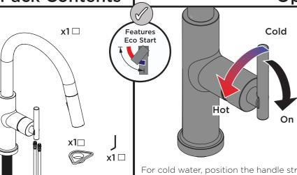
For cold water, position the handle straight upwards. To increase the temperature, turn the handle to the left.
