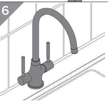
Turn on the water supply. Check all joints and connections for any leaks.
