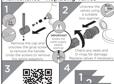
Reverse the steps to replace the valves and handles.
