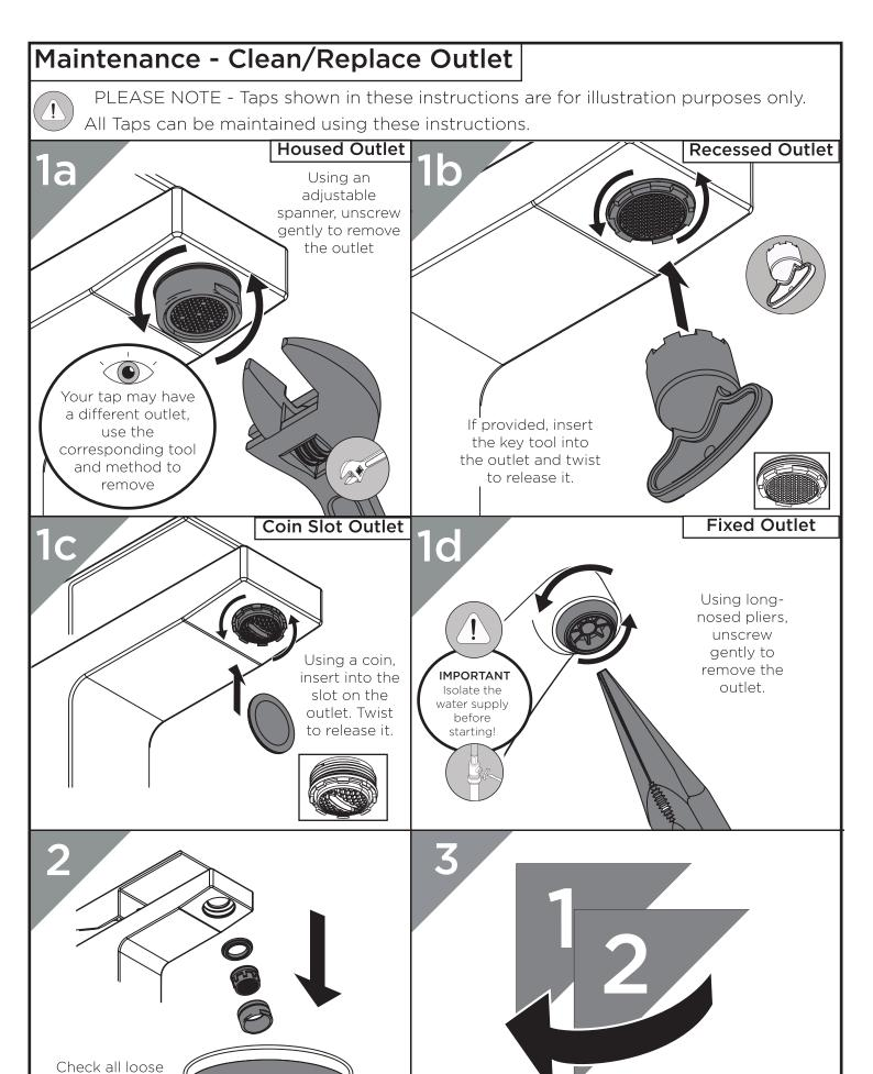
parts for any damage, then soak using a suitable solution to de-scale
