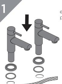
Feed the tap body through the bath/basin and ensure plinth and plinth seals are in place.
