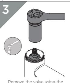
Remove the valve using the tool required for your tap. Check any seals and O-rings for damage. Replace valve if necessary.
