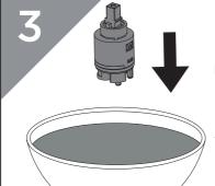
Place cartridge in a suitable solution and soak until fully de-scaled.
