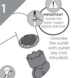
Place outlet parts a suitable solution and soak until fully de-scaled.
