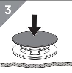
Push the centre down to close the waste. Push again to open and release contents of basin.
