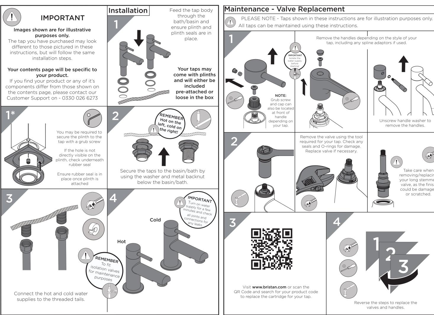
Remove the handles depending on the style of your tap, including any spline adaptors if used. Unscrew handle washer to remove the handles. Take care when removing/replacing your long stemmed valve, as the finish could be damaged or scratched. Reverse the steps to replace the valves and handles.
