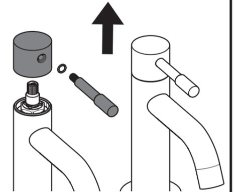
Unscrew handle washer to remove the handles.
