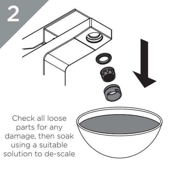
Check all loose parts for any damage, then soak using a suitable solution to de-scale
