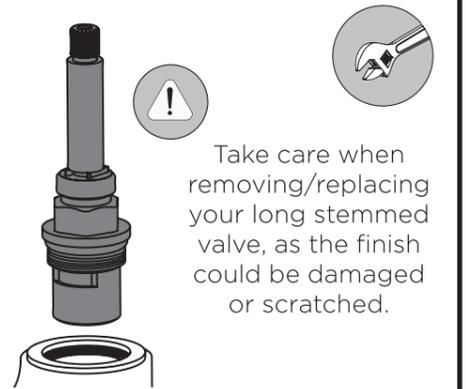
Take care when removing/replacing your long stemmed valve, as the finish could be damaged or scratched.
