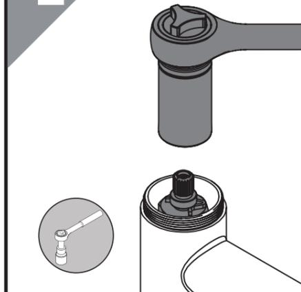
Remove the valve using the tool required for your tap. Check any seals and O-rings for damage. Replace valve if necessary.
