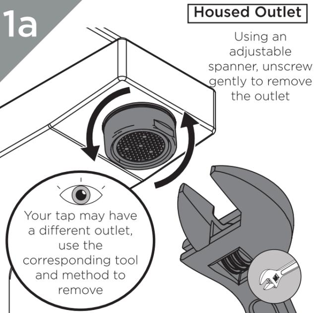
Your tap may have a different outlet, use the corresponding tool and method to remove
