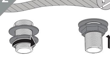
To secure the taps to the bath, use a box spanner to tighten the metal backnuts underneath ensuring the washer is correctly positioned in between the backnuts and the bath
