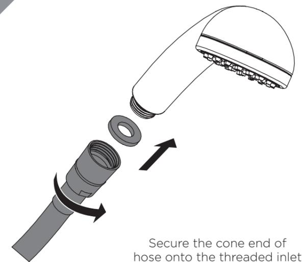
Secure the cone end of hose onto the threaded inlet connection of the handset, ensuring the washer is in place, before tightening
