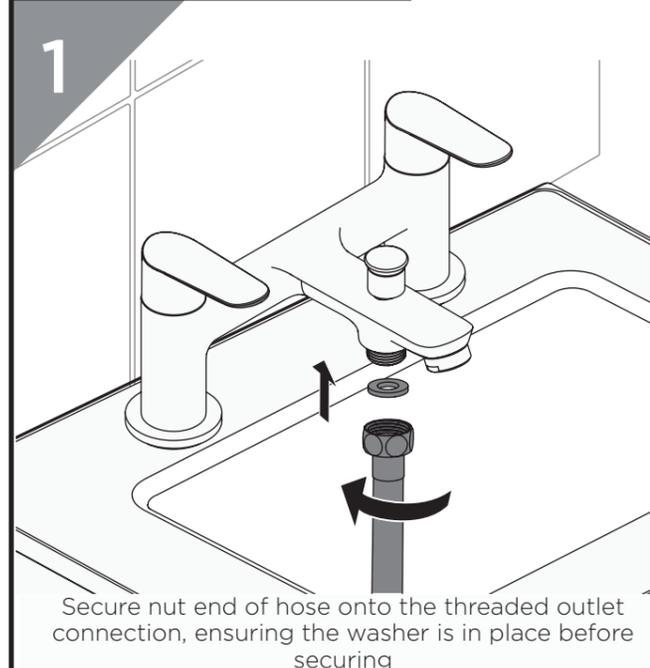
Secure nut end of hose onto the threaded outlet connection, ensuring the washer is in place before securing
