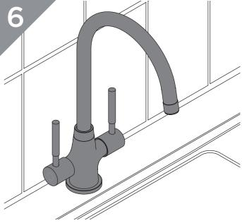
Turn on the water supply. Check all joints and connections for any leaks.
