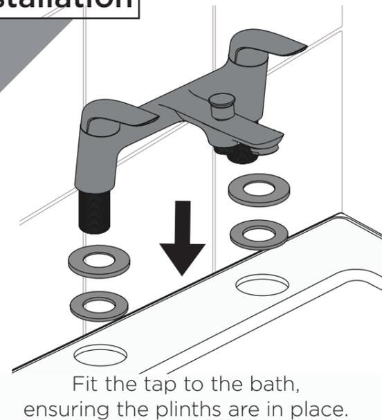
Fit the tap to the bath, ensuring the plinths are in place.
