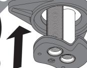
Feed the base through the sink hole from the top.
