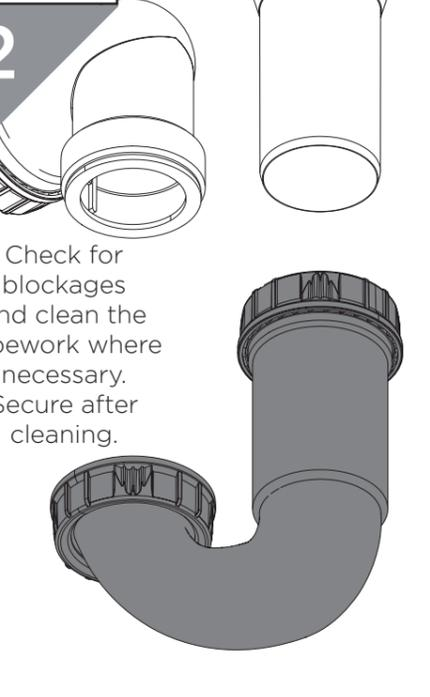
Check for blockages and clean the pipework where necessary. Secure after cleaning.
