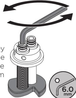
Turn the hexagonal key anti-clockwise to remove the back nut from the EasyFit Base.
