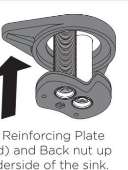
Feed the Reinforcing Plate (if required) and Back nut up to the underside of the sink.
