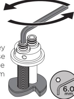
Turn the hexagonal key anti-clockwise to remove the back nut from the EasyFit Base.
