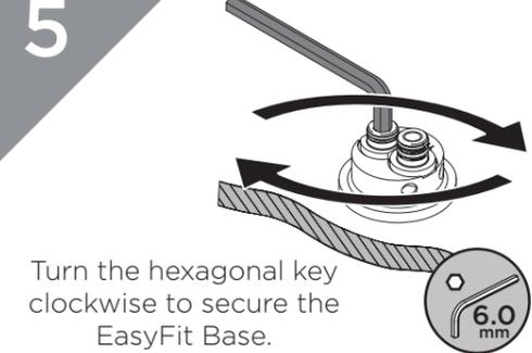
Turn the hexagonal key clockwise to secure the EasyFit Base.
