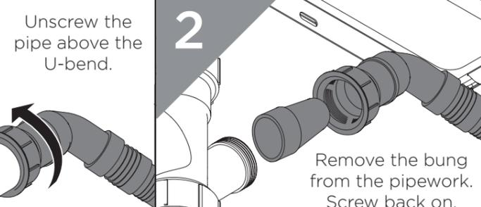
Remove the bung from the pipework. Screw back on.
