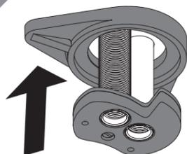
Feed the Reinforcing Plate (if required) and Back nut up to the underside of the sink.
