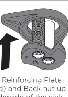
Feed the Reinforcing Plate (if required) and Back nut up to the underside of the sink.
