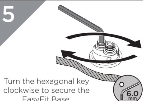
Turn the hexagonal key clockwise to secure the EasyFit Base.
