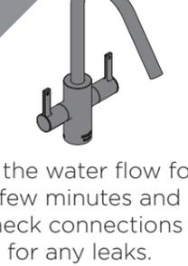
Let the water flow for a few minutes and check connections for any leaks.
