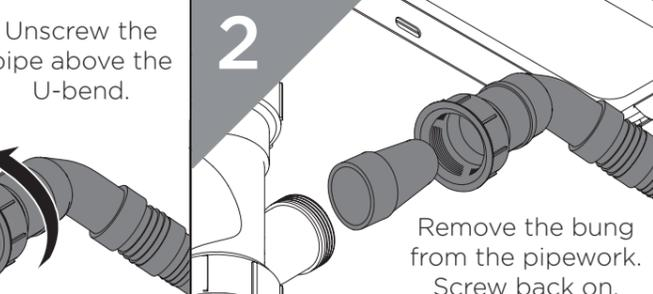
Remove the bung from the pipework. Screw back on.
