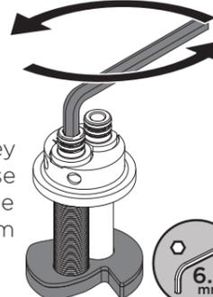
Turn the hexagonal key anti-clockwise to remove the back nut from the EasyFit Base.
