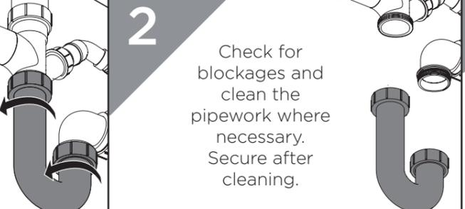
Check for blockages and clean the pipework where necessary. Secure after cleaning.
