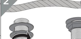
To secure the taps to the bath, use a box spanner to tighten the metal backnuts underneath ensuring the washer is correctly positioned in between the backnuts and the bath.
