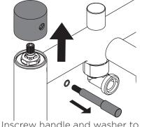
Unscrew handle and washer to remove the handles.
