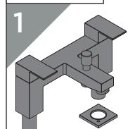
Feed the tap body through the plinths and ensure rubber plinth seals are in place.
