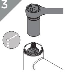
Remove the valve using the tool required for your tap. Check any seals and O-rings for damage. Replace valve if necessary.
