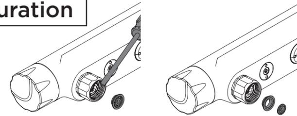
Use a thin flat blade screwdriver, or similar tool, to carefully prise the flow regulators from both inlets.
