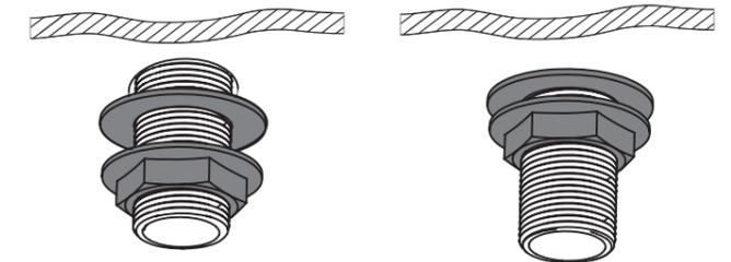
Secure the taps to the bath by using the washer and metal backnut below the bath.
