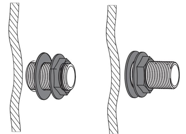
Secure the taps by using the washer and metal backnut behind the wall.
