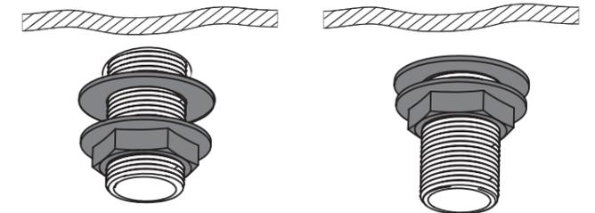
Secure the taps to the bath by using the washer and metal backnut below the bath.
