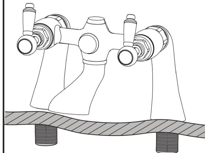
Connect the hot and cold water supplies to the threaded tails.
