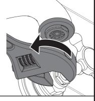
Unscrew the valve using an adjustable spanner.
