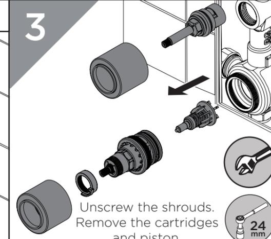
Unscrew the shrouds. Remove the cartridges and piston.
