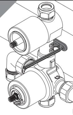
Install suitable batons (if required) into the cavity. Mark the position of the valve; drill and plug holes to suit.
