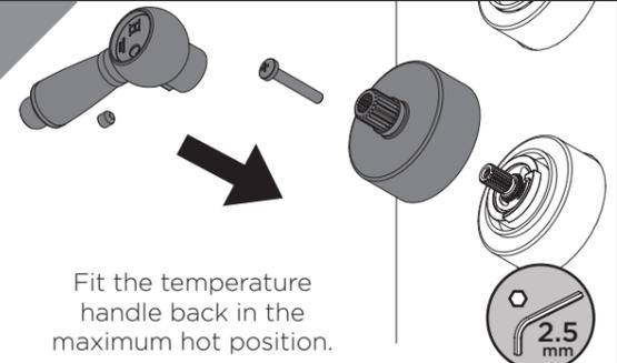
Fit the temperature handle back in the maximum hot position.
