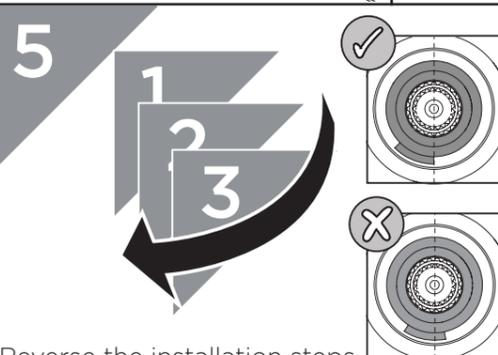
Reverse the installation steps, ensuring the temperature stop is aligned correctly.
