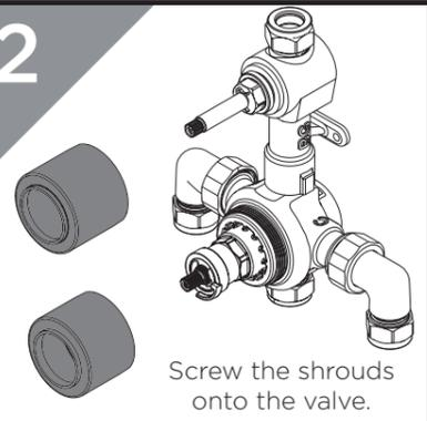
Screw the shrouds onto the valve.
