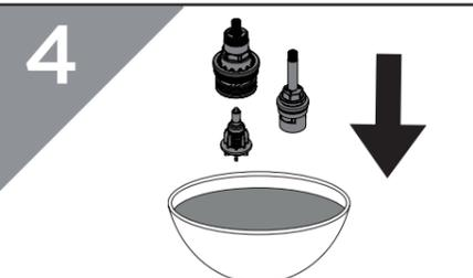
Remove any O-rings and soak all components in de-scaler and wash off in clean water. Examine all seals and replace if needed. Use WRAS approved silicon based grease on all seals.
