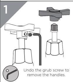
Remove the screw. spline adaptor and valve shrouds.
