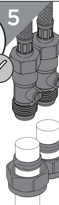
Connect the hot and cold water connections.
