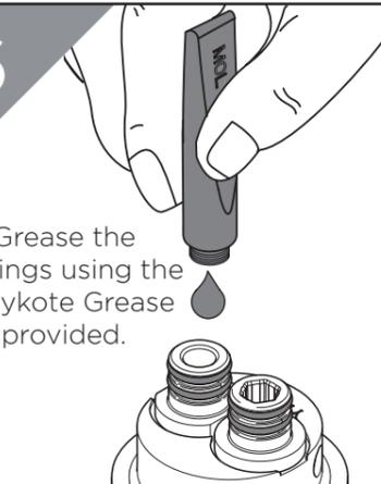
Grease the O-Rings using the Molykote Grease provided.
