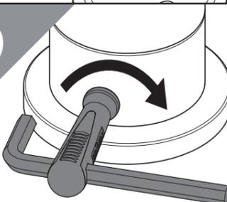
Thread the hexagonal key through the EasyFit tool and tighten the grub screws with an extra 1/2 turn.
