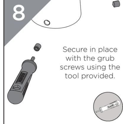
Secure in place with the grub screws using the tool provided.
