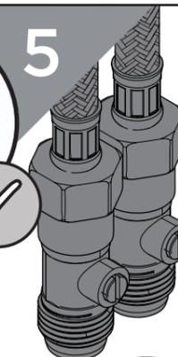
Connect the hot and cold water connections.
