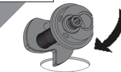
Feed the base through the sink hole from the top.
