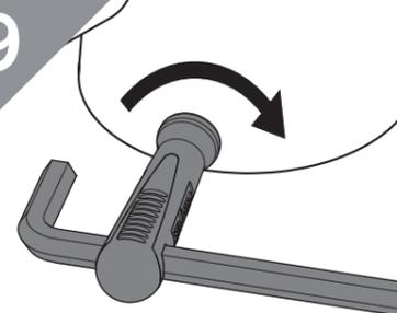
Thread the hexagonal key through the EasyFit tool and tighten the grub screws with an extra 1/2 turn.
