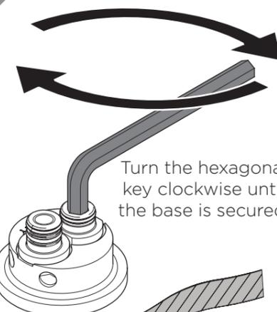
Turn the hexagonal key clockwise until the base is secured.
