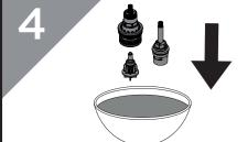
Remove any O-rings and soak all other components in de-scaler; wash off in clean water. Examine all seals and replace if needed. Use WRAS approved silicon based grease on all seals.
