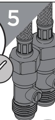
Connect the hot and cold water connections.
