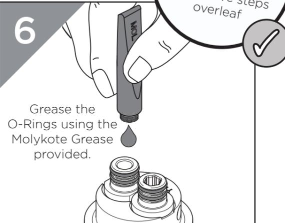
Grease the O-Rings using the Molykote Grease provided.
