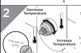
Turn the spindle to increase or decrease the temperature. Check the temperature and adjust until you achieve the desired result.
