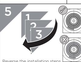
Reverse the installation steps, ensuring the temperature stop is aligned correctly.
