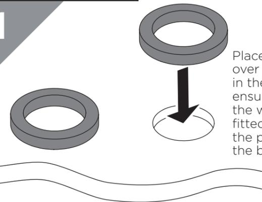
Place the plinths over the holes in the bath ensuring that the washers are fitted between the plinths and the bath.
