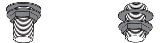
Secure the body to the bath by using the washer and metal back nut below the bath. Tighten the back nut onto the threaded tails.
