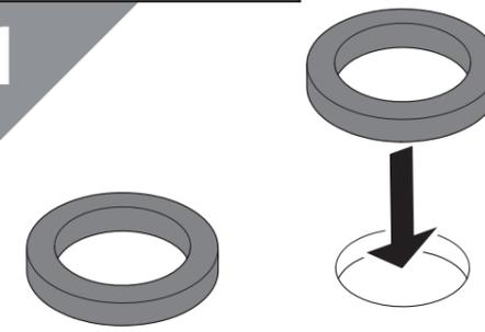
Place the plinths over the holes in the bath ensuring that the washers are fitted between the plinths and the bath.
