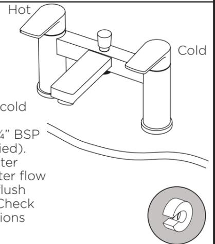
Connect the hot and cold water supplies to the threaded tails using 3/4" BSP connector (not supplied). Turn on the mains water supply letting the water flow for a few minutes to flush through the system. Check all joints and connections for any leaks.
