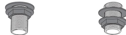
Secure the body to the bath by using the washer and metal backnut below the bath. Tighten the backnut onto the threaded tails.
