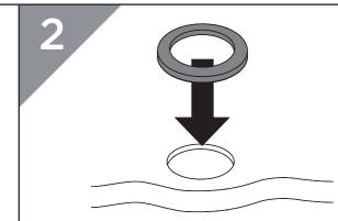
Place the plinth over the hole in the basin ensuring that the washer is fitted between the plinth and the basin.
