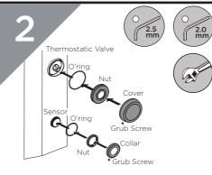
Loosen the sensor/valve grub screws. remove the collar/ cover, remove the nuts and the O-rings from the shower panel.
