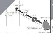
Fit the O'ring into the wall nut and secure wall nut onto head post. Push shower head onto head post ensuring the anti-rotation pin is located in the anti-rotation pin hole and secure with grub screws.
