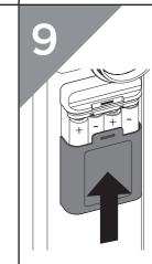
Insert 4 x Alkaline LR6 1.5 V AA (preferably 2000mAh) batteries to the battery pack. Slide the battery pack cover up.
