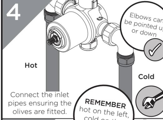
Connect the inlet pipes ensuring the olives are fitted.
