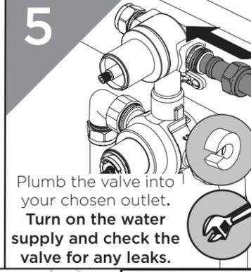
Plumb the valve into your chosen outlet. Turn on the water supply and check the valve for any leaks.
