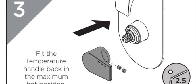
Fit the temperature handle back in the maximum hot position.
