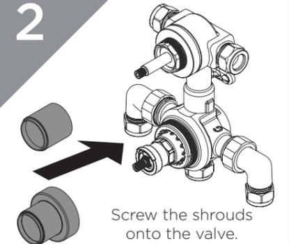
Screw the shrouds onto the valve.
