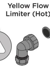
Remove the inlet elbows and filters. Remove the plastic inserts from the valve inlets and insert the flow regulators. Replace the elbows, ensuring the filters are fitted.
