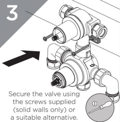
Secure the valve using the screws supplied (solid walls only) or a suitable alternative.
