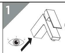
Look underneath the tap body to observe fixing kit rod(s) and tail inlet positions.
