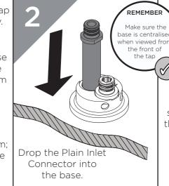
Ensure flat area of the plain inlet connector sitting flush adjacent to threaded inlet connector
