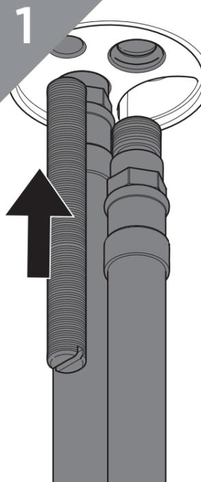
Screw in the flexible tails by hand. **DO NOT OVERTIGHTEN.**
