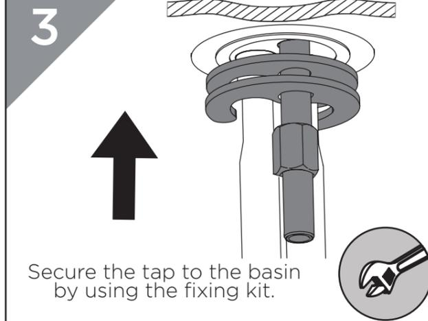
Secure the tap to the basin by using the fixing kit.
