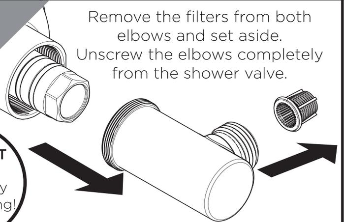
Remove the filters from both elbows and set aside. Unscrew the elbows completely from the shower valve.
