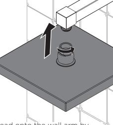
Screw the shower head onto the wall arm by HAND ONLY. Turn on the water supply and check all joints and connections for any leaks.
