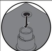
Ensure the filter washer is correctly inserted into the fixed head.
