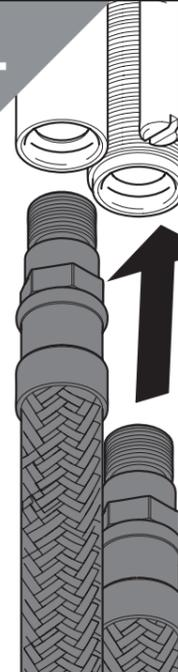
Screw the flexible tails into the base.
