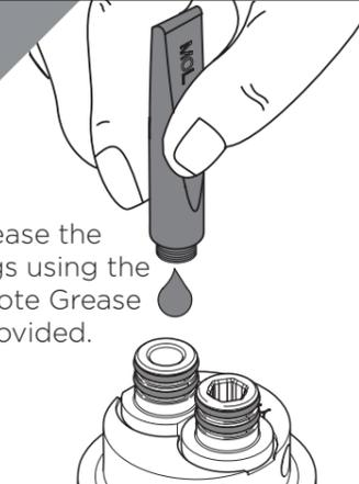
Grease the O-Rings using the Molykote Grease provided.
