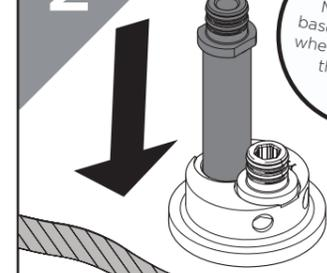
Drop the Plain Inlet Connector into the base.
