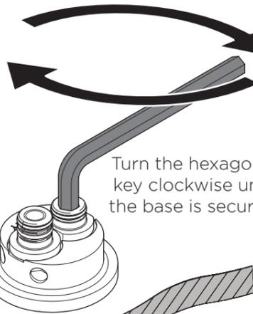
Turn the hexagonal key clockwise until the base is secured.
