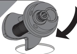
Feed the base through the sink hole from the top.
