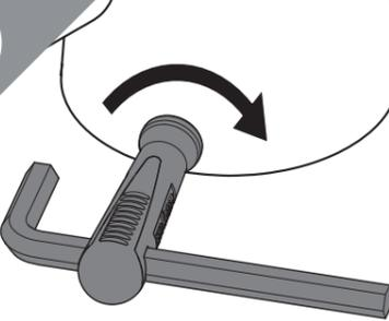
Thread the hexagonal key through the EasyFit tool and tighten the grub screws with an extra 1/2 turn.
