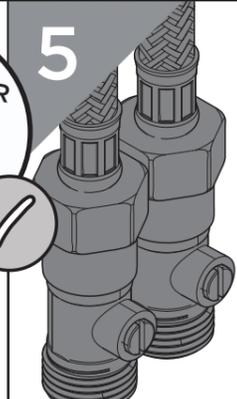
Connect the hot and cold water connections.
