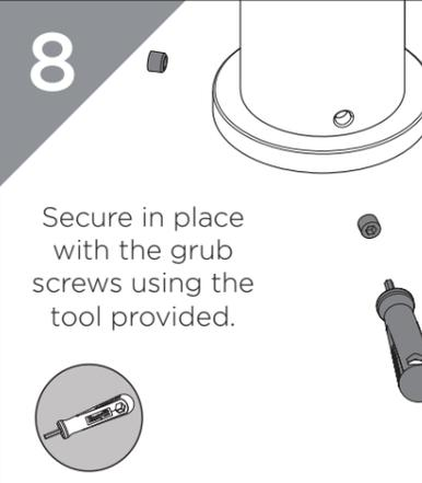
Secure in place with the grub screws using the tool provided.
